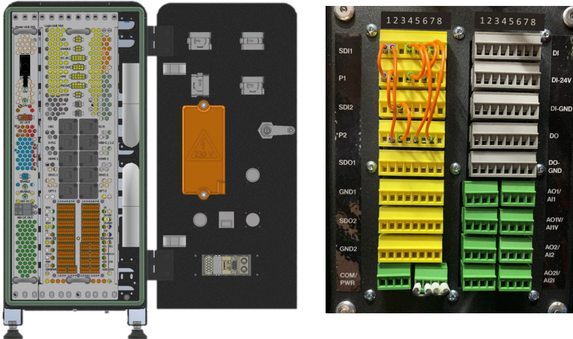
Fig. 21: Customer I/O board factory default electrical bridges
