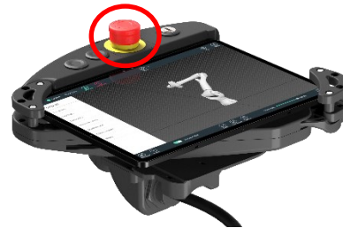
Fig. 37: Emergency stop button at Teach Pendant
